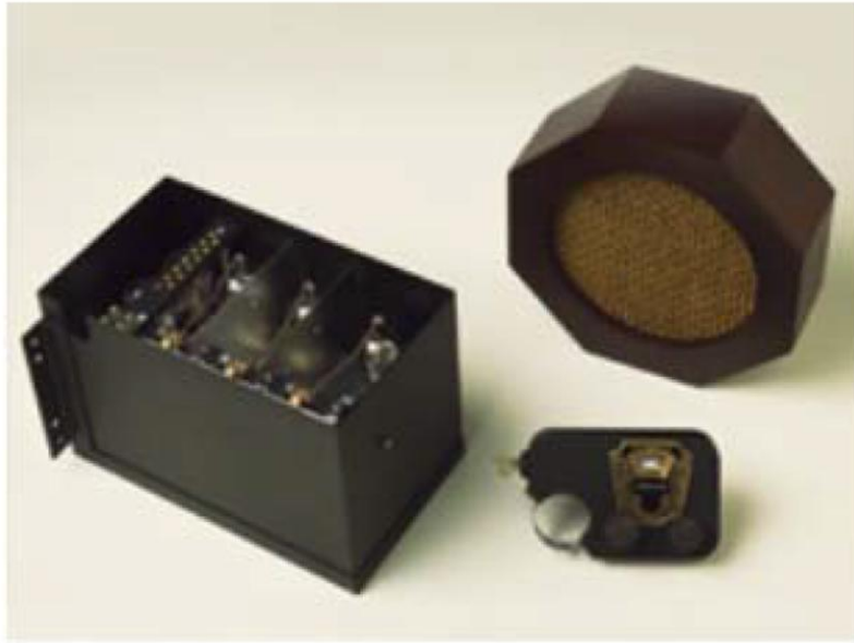
Reproduction of a Motorola 5T71, included (left to right) the receiver, tuning control, speaker.
