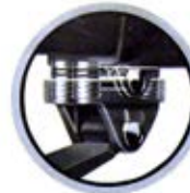
Four coiled springs recessed at the top of the ball beam spring assembly, insured results in steering safety and control.
