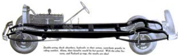
The steering gear is exclusively Packard in design and manufacture and fitted with a combination of ball and roller bearings to insure against fatigue in parking and in traffic operation.
