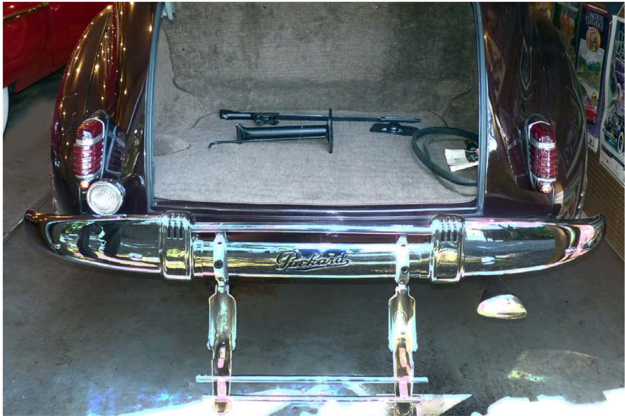
The bumper guard drops down for access to the trunk compartment
