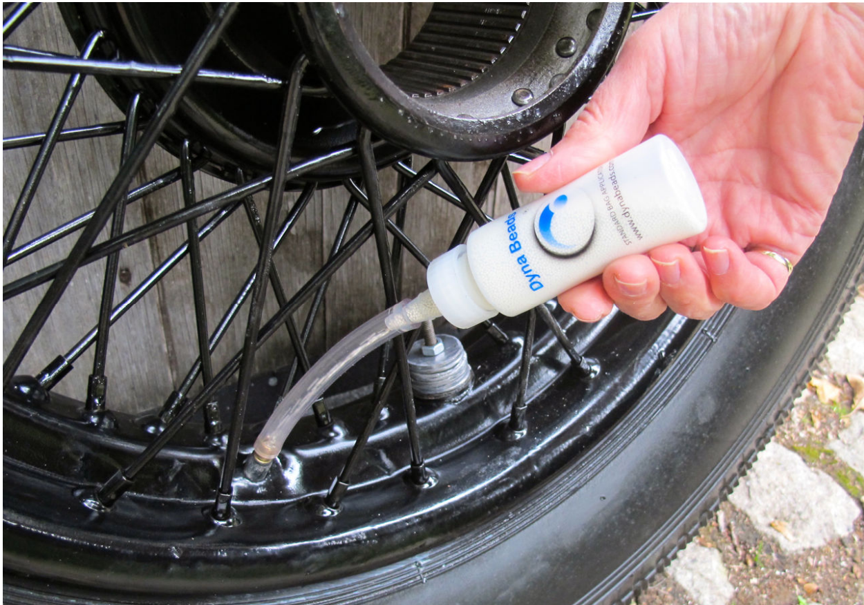
3 Ceramic beads being injected using an applicator.
