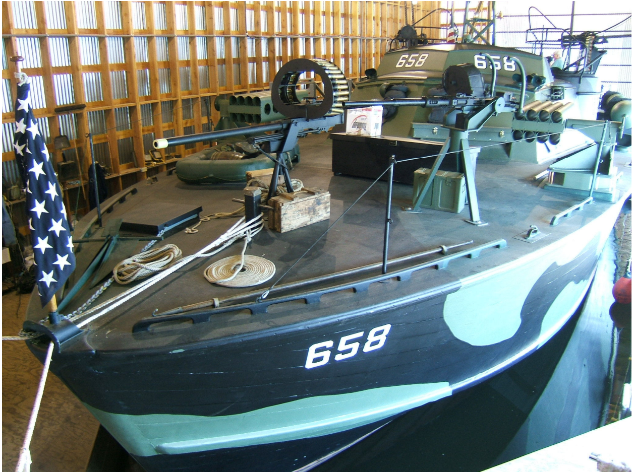
Bow armament on PT 658, a 37mm Oldsmobile M9 auto cannon center front, an M4 20mm Oerlikon auto cannon right and 8 5" rocket launch tubes on either side.
