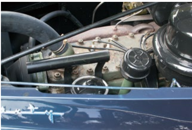
View of the driver's side of the engine compartment. Packard's 356 Cid, 9 main bearing engine with hydraulic valve tappets produced 160 bhp. It was widely regarded as the ultimate straight eight automobile engine with its smooth, quiet power.
