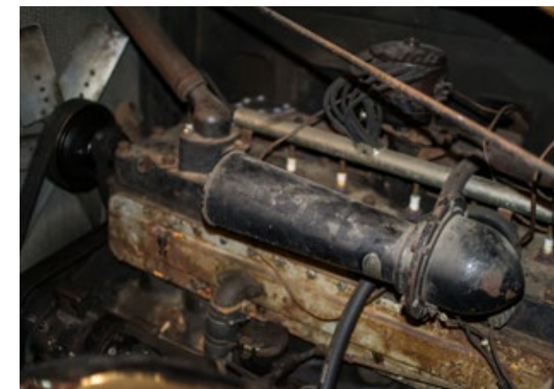
A hallmark of Pierce-Arrow's engineering excellence was its silk-smooth 9 main bearing straight-eight 385 CID engine generating 132 BHP.
